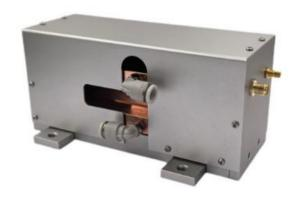
The key parameter of AOM is the rise/fall time, which defines the achievable "speed" or amplitude modulation bandwidth of the modulation. The rise/fall time is proportional to the beam diameter within the modulator. Therefore, in order to obtain a fast rise time, it is necessary to control the diameter of the incident laser beam.
